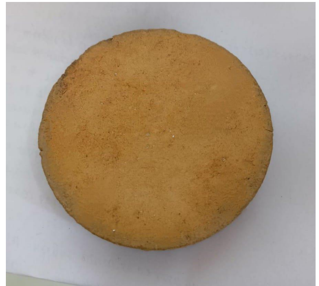
Figure 3: Ceramic Membrane after sintering in muffle furnace
